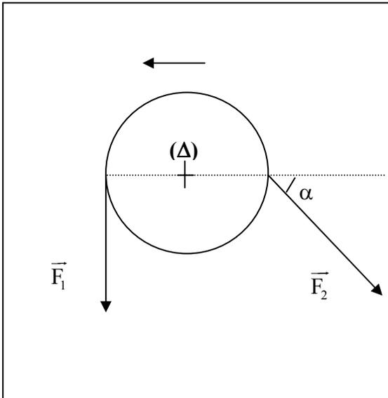
$F_1 = 10 \text{ N}$  ;  $F_2 = 20 \text{ N}$  et  $\alpha = 45^\circ$
