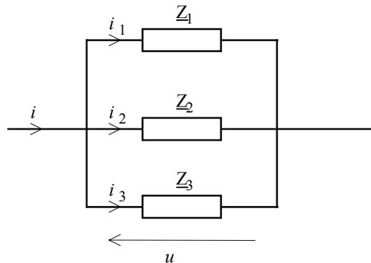
$$\underline{I} = \underline{I}_1 + \underline{I}_2 + \underline{I}_3 = (\underline{Y}_1 + \underline{Y}_2 + \underline{Y}_3) \underline{U}$$
