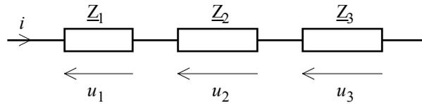
$$\underline{U} = \underline{U}_1 + \underline{U}_2 + \underline{U}_3 = (\underline{Z}_1 + \underline{Z}_2 + \underline{Z}_3) \underline{I}$$
